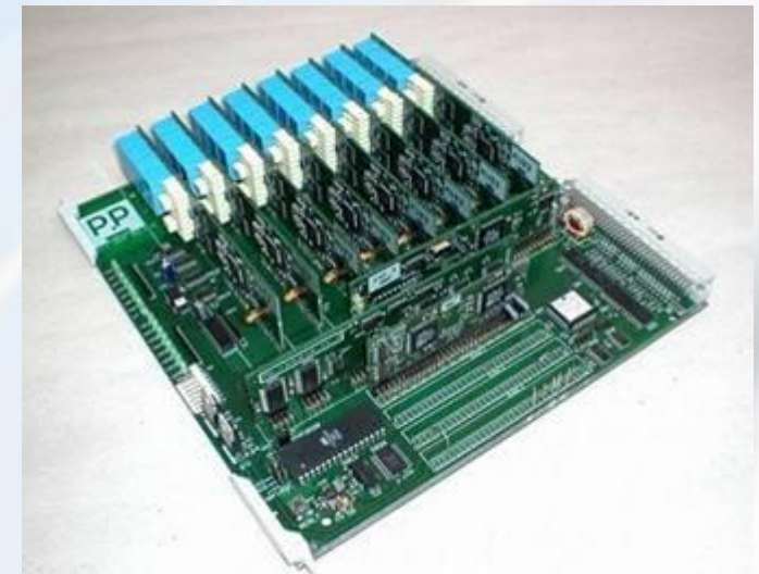
19" plug-in board - interface 220 x 233 mm FRONT, BACK
